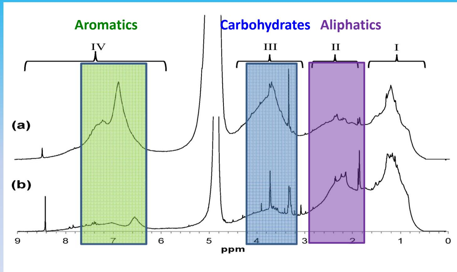
■ Aromatic and carbohydrate components represented up to 70% of deep bog DOM but comprised a much smaller proportion of deep fen DOM
